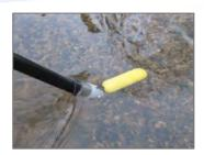
The Aqua-Data FloStick RC4 Water Velocity Meter is a standalone instrument comprising velocity probe, wading rod and display housing, all in a single integrated package. It uses the Faraday principle of electromagnetic induction and advanced analogue and digital electronics to offer an accurate, robust and low-cost method of measuring water velocity, and logging data for later analysis.
