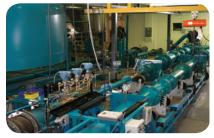
Our Hemet, California factory boasts a robust Calibration Test Lab that enables production of the most accurate and precise flow instrumentation. The test facility utilizes three gravimetric systems and two volumetric systems providing accuracy and calibration tests of flow meters from 1/2 to 20-inch diameter, with flow rates up to 4,000 gpm.
