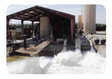
Our large volume test facility is located in Porterville, California. This facility is one of the world's largest volumetric test facilities owned by a meter manufacturer, and it offers accuracy and calibration tests of flow meters from 3 to 72-inch diameter, with flow rates up to 60,000 gpm.
