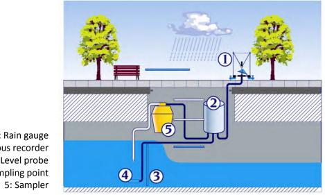
1: Rain gauge 2: Octopus recorder 3: Level probe 4: Sampling point
