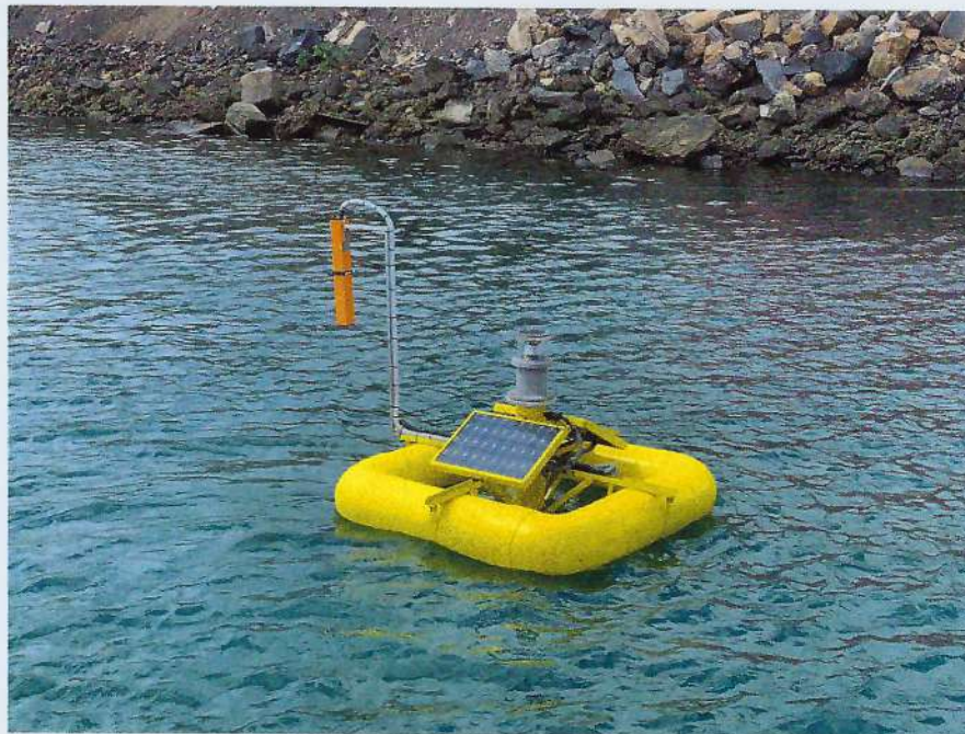
Hydrocarbon sheens will tend to surface once entering laminar flow areas in rivers and streams. Here is where early detection is most critical for an appropriate oil spill response.
