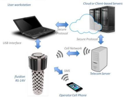
The RS-14V system uses a wireless communication protocol based on the cellular network for both system configuration and data management. The system can be fully configured from a mobile phone using intuitive SMS-based commands. Communication is established via the cellular network. In case there is no cell coverage in the installation area, the system can be pre-configured from a PC via the USB interface.
