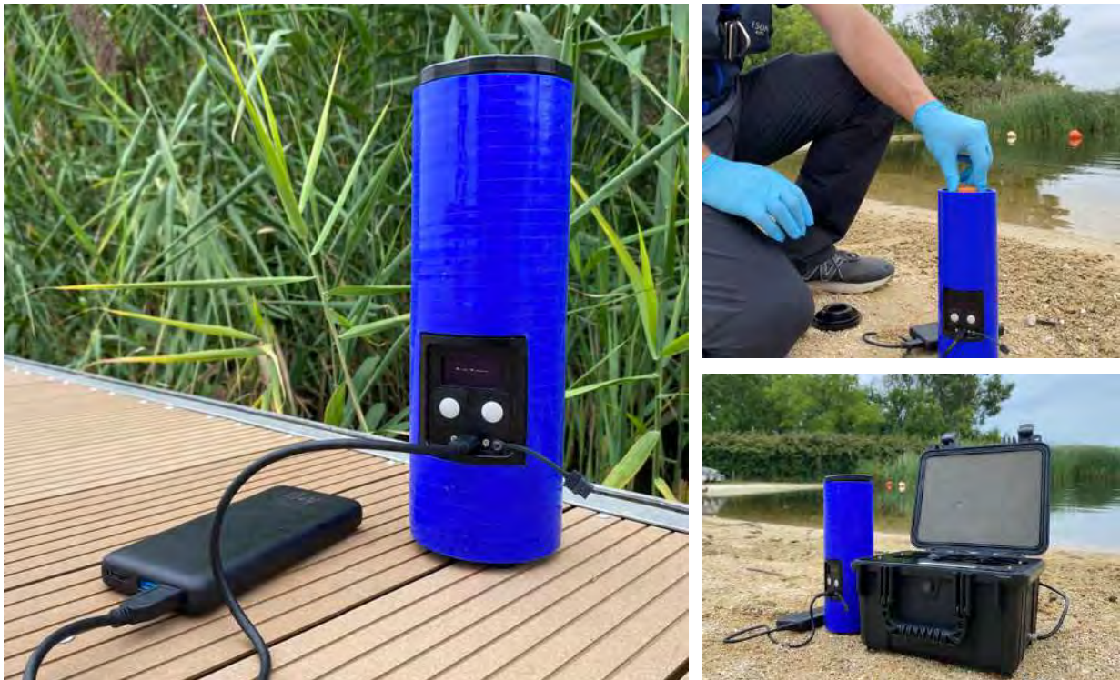
Left: ALERT One performing a measurement at an urban recreational site, powered by a portable battery pack.
