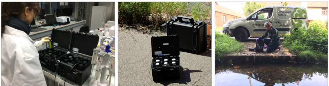
Left: ALERT LAB being used in a water quality analysis laboratory. Middle: The equipment during a field operation, analyzing six samples simultaneously. Right: ALERT LAB as used by regulatory agency agent in the field.
